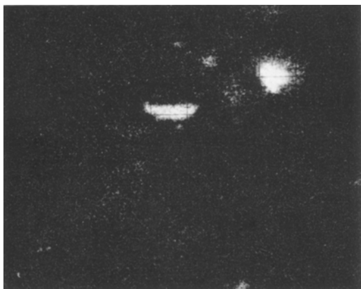
Figure 1b Magnesium X-ray scan for unexposed neoprene.
