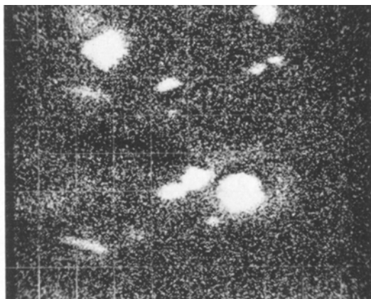
Figure 2b Magnesium X-ray scan for neoprene exposed to 10% magnesium sulphate solution for 20 min.
